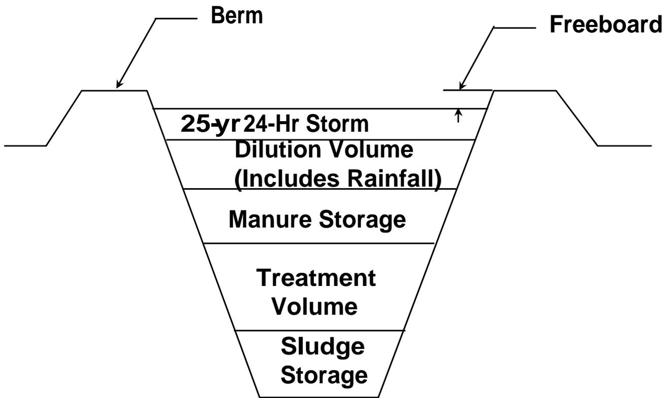
**Figure 1. Capacities that must be included in a proper lagoon design.**
