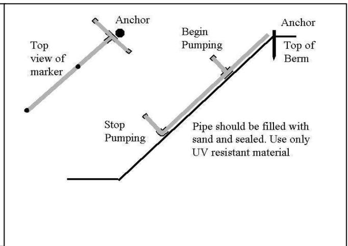
**Figure 4. Example of Sloped pump-down marker in earthen impoundment**
