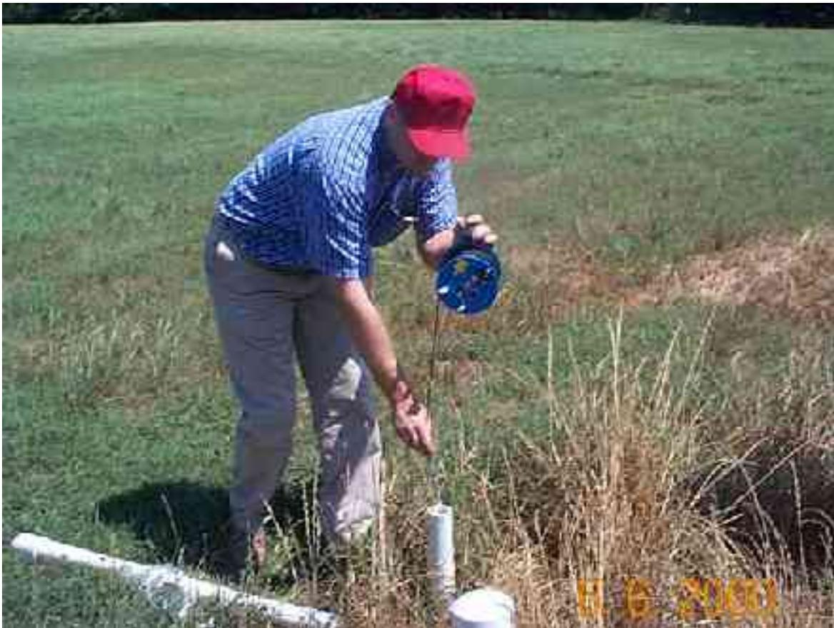
*Figure 12. Measuring the depth to groundwater*
